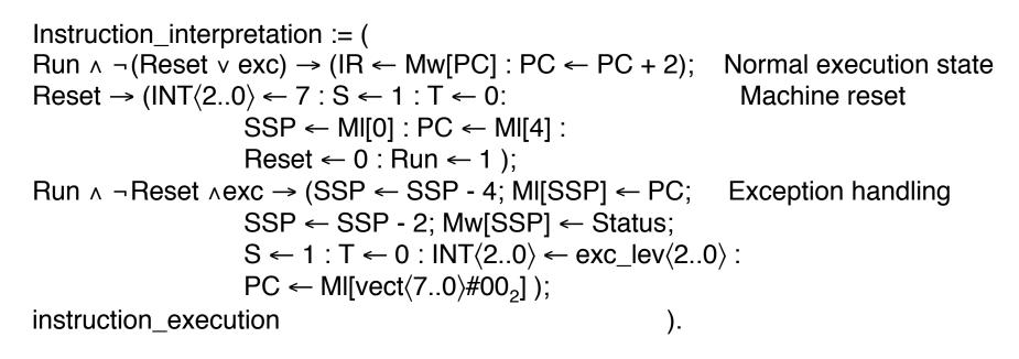
Reset starts the computer with a stack pointer from location 0 at the address from location 4
