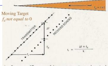
4. Frequency difference,  $\Delta f$ , between transmitter and received echoes is reduced by target's doppler frequency,  $f_d$ . To find transit time,  $f_d$  must be added to  $\Delta f$ .
