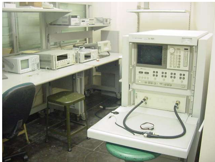
(b) Network Analyzer 8350 and other microwave equipment.
