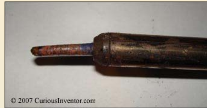
Corroded pin repels solder
