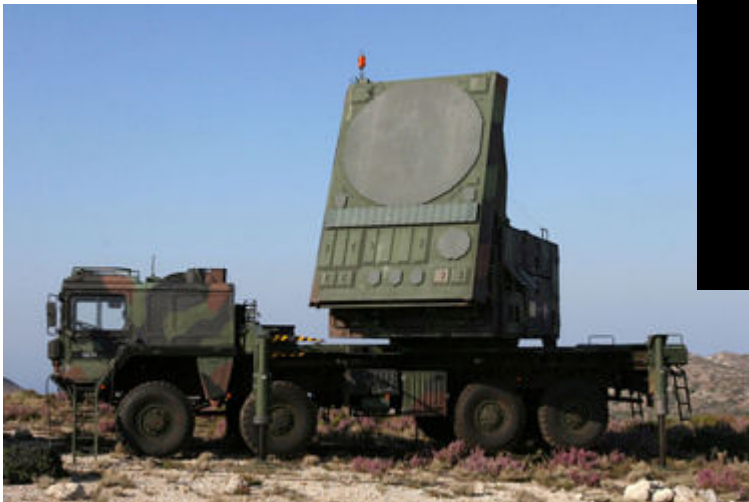
Phased array antennas
