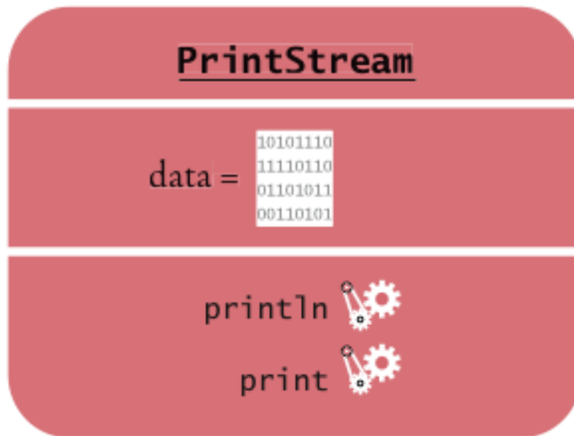
Figure 4 Representation of the System.out Object
