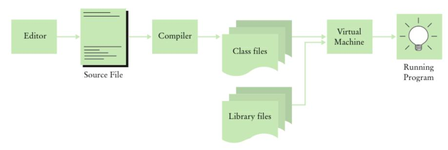
Figure 10 From Source Code to Running Program
