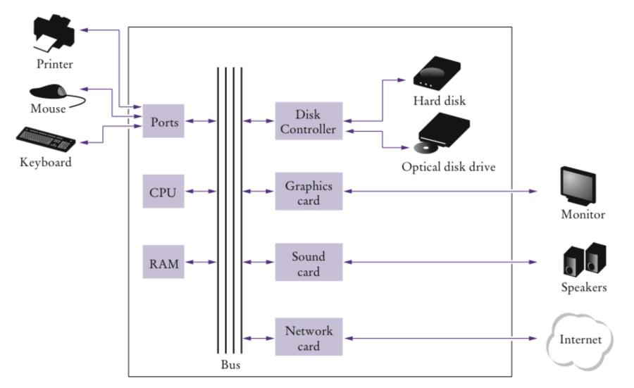
Figure 5 Schematic Diagram of a Computer
