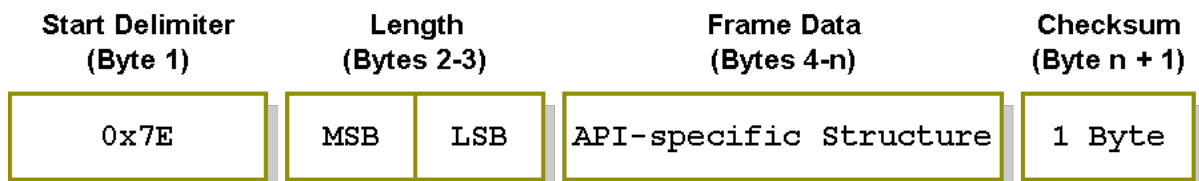
Figure 4.3 General XBee API Frame Structure
