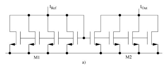
$$\left(\frac{\delta I_{out}}{I_{out}}\right)^2 = \frac{1}{n} \left[ \left(\frac{\delta W}{W}\right)^2 + \left(\frac{\delta L}{L}\right)^2 \right] + K$$
