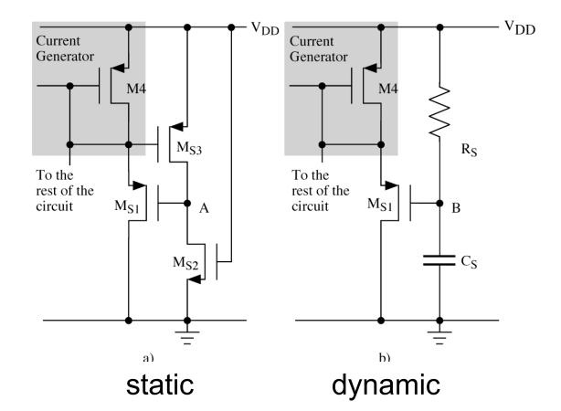
Monitor if the current is zero and inject a current that starts the circuit.
