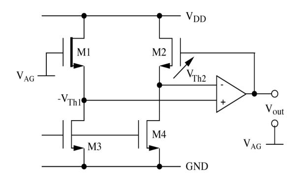
M1 and M2 have different threshold (enhancement and depletion or enhancement and enhancement)
