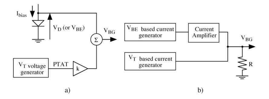
a) implementation adding voltagesb) implementation adding currents and transforming current into voltage
