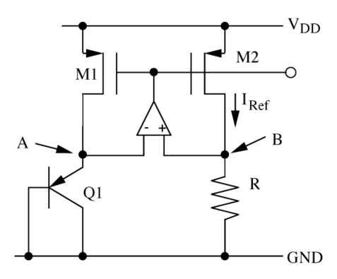
The voltage across the resistance and the diode voltage are made equal by the feedback loop action.
