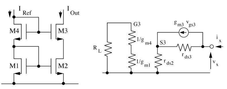
It increases the output resistance without feedback loop. It has the same resistance of the cascode load.
