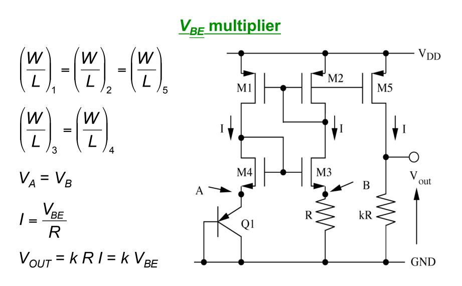
$V_{OUT}$  has a negative temperature coefficient
