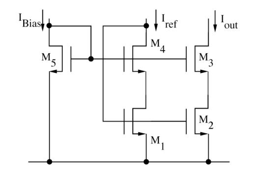
M1 = M2; M3 = M4 therefore  $I_{out} = I_{ref}$ To properly work, we must impose  $V_{DSsatM4} < V_{Th1}$
