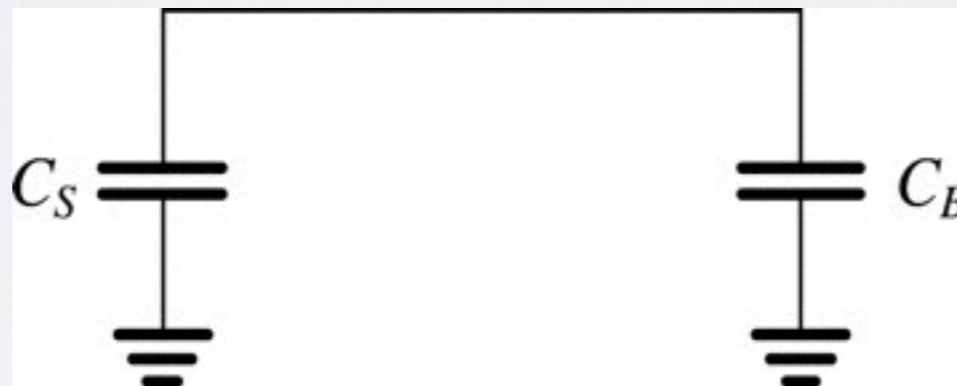
Figure 16.19 When the voltage of the selected word line is raised, the transistor conducts, thus connecting the storage capacitor C_S to the bit-line capacitance C_B .
