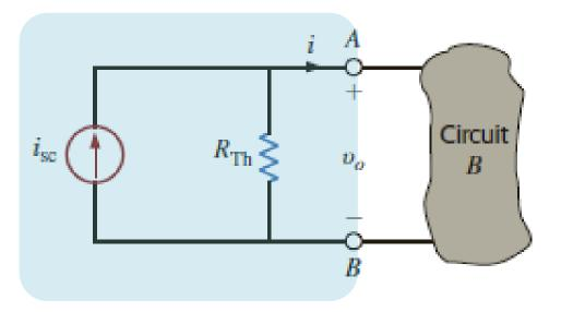
Thevenin and Norton Equivalent circuits are equivalent... hence source transformation is possible remembering
