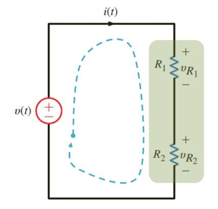
$v_{R_1} = ?$  $v_{R_{2}} = !$ • KVL:  $v(t) = v_{R_1} + v_{R_2}$ • Ohm's:  $v_{R_1} = R_1 \cdot i(t)$   $v_{R_2} = R_2 \cdot i(t)$   $\therefore i(t) = \frac{v(t)}{R_1 + R_2}$  $\therefore v_{R1} = \frac{R_1}{R_1 + R_2} \cdot v(t)$  $v_{R2} = \frac{R_2}{R_1 + R_2} \cdot v(t)$
