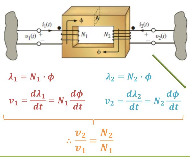
Assuming an ideal magnetic core with infinite permeability...
