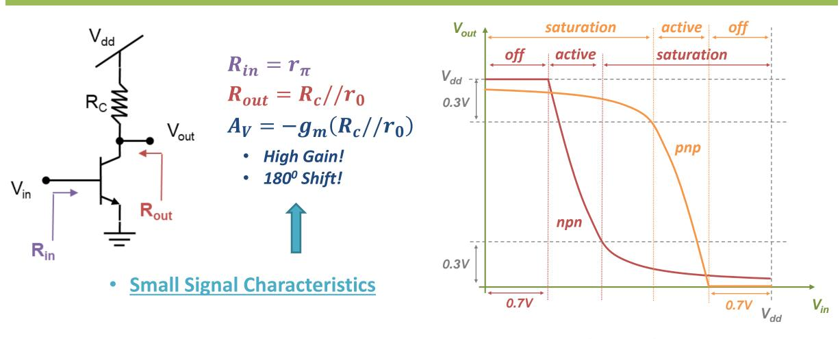
Common Emitter<sub>npn</sub> vs Commom Emitter<sub>pnp</sub>?  $A_{v_npn} = A_{v_pnp}$
