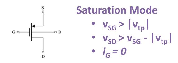
$V_{ov} = V_{SG} - |V_{tp}|$
