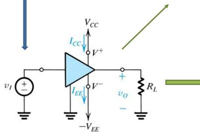
$$V_{out}(t) = A_V \cdot V_{in}(t)$$
