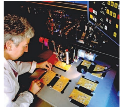
Troubleshooting an electronic circuit board.
