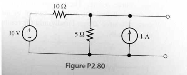
2. Find the Thevenin and Norton equivalent circuits for the circuit shown in Figure P2.88.
