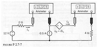
**P 2.7-7** Find the power absorbed by the CCVS in Figure P 2.7-7.
