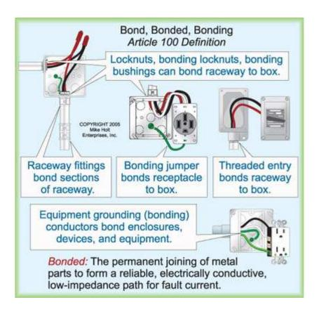
Effective ground-fault current path [250.2]. An intentionally constructed, permanent, low-impedance conductive path designed to carry fault current from the point of a ground fault on a wiring system to the electrical supply source. The effective ground-fault current path is intended to help remove dangerous voltage from a ground fault by opening the circuit overcurrent protective device.
