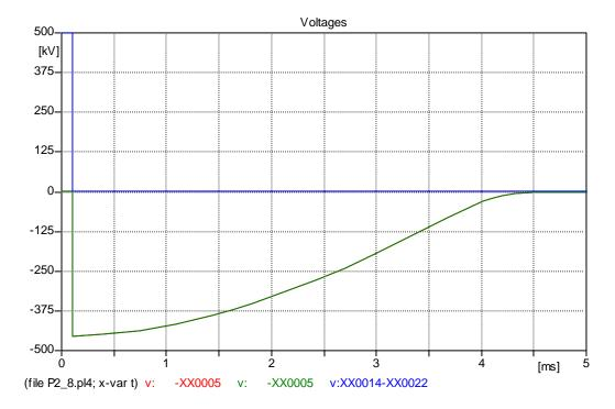
This is the result at time equals infinity in the simulated circuit. The voltage will drop down to zero since there is no forcing function to re-energize the circuit.
