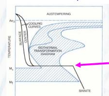
Austempering: Used in order to produce a 100% bainitic structure that has a high yield strength. Note that the isothermal treatment is conducted a few degrees above M<sub>S</sub>. Why?
