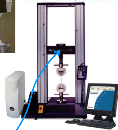
5860 Instron® Model with 50kN capacity
