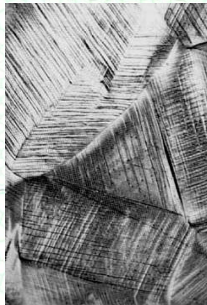
Slip lines in a polycrystalline copper sample
