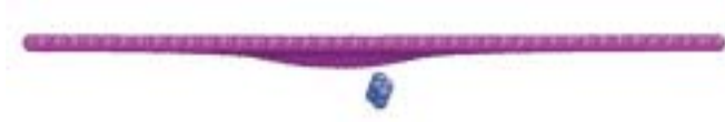
Fig. 5 Atomistic simulation result for indentation of Al with a spherical indenter tip, illustrating the nucleation of a dislocation beneath the indented surface 57 . Only miscoordinated atoms are visible, revealing the position of the surface (colored pink and bowed out under the load of the indenter) as well as the first crystal defect that formed at the yield point (colored in blue). (Reprinted courtesy of K. J. Van Vliet, Massachusetts Institute of Technology and with permission from 57 . © 2005 American Physical Society.)
