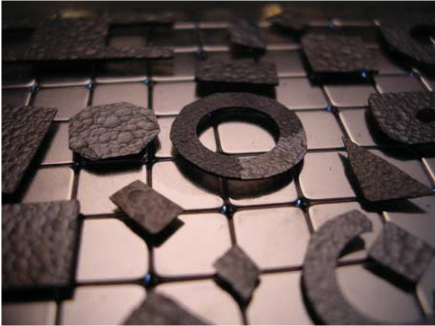
Figure 5. Pieces of pyrolitic graphite, cut into various shapes, hover intriguingly. In this demonstration, about 120 objects in all floated above a base of permanent magnets. A powered device that could lift an equally large number and variety of objects using active feedback would be a significant engineering challenge to design and build, whereas this simple system of passive, diamagnetic levitation is straightforward to assemble. (Courtesy of the author.)
