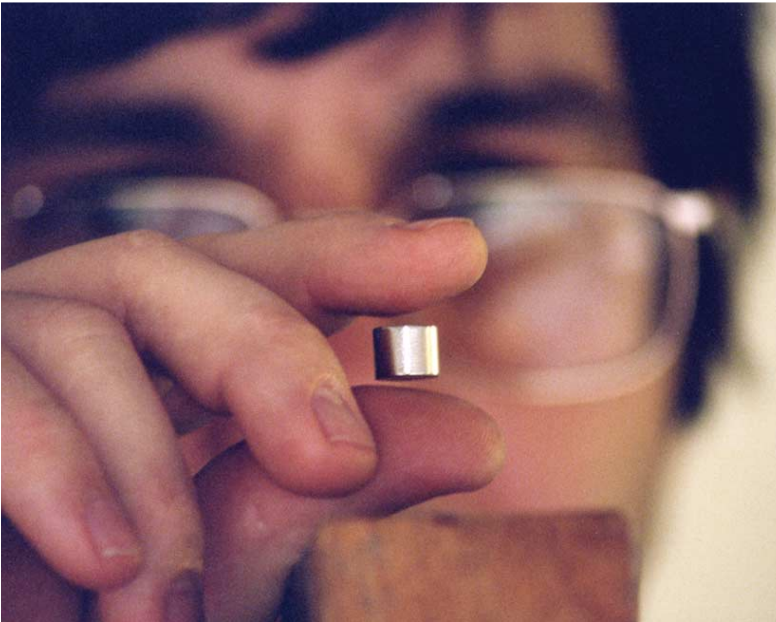
Figure 1. Floating between thumb and forefinger, this small magnet demonstrates the surprising phenomenon of diamagnetic levitation. In this experiment, a powerful superconducting magnet located on the floor above provides the lifting force necessary to counter gravity. Having one magnet lift another in that way is, however, inherently unstable, as anyone who has played with a pair of refrigerator magnets can attest. In this case the weak diamagnetism of the investigator's fingers provides a modest repulsive force when the small magnet approaches, stabilizing the levitation. The author and his engineering colleagues have used this same principle to design devices intended for commercial application. (Courtesy of Andre Geim, University of Manchester.)
