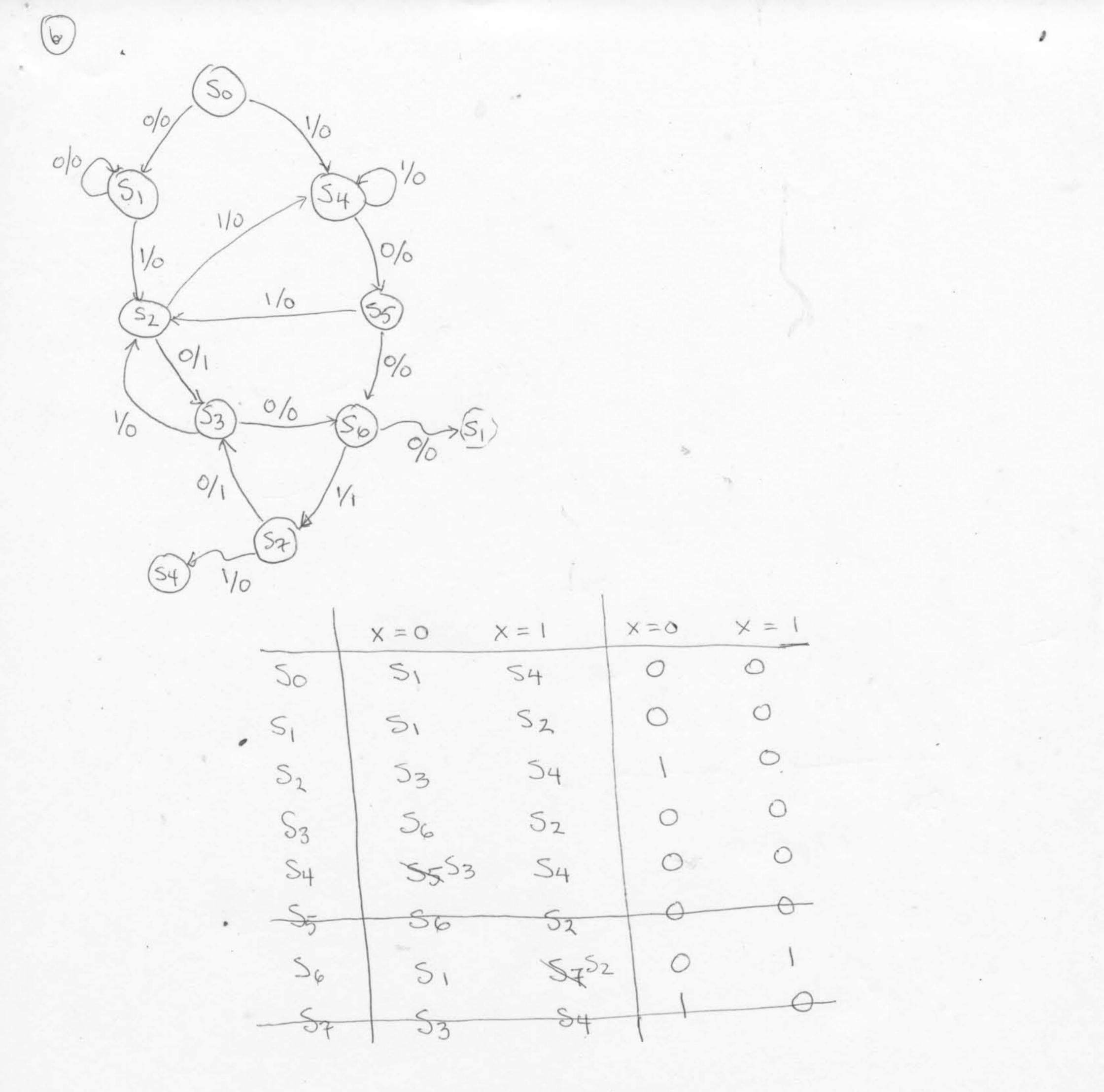
St is equivalent to S2 S5 is ..... 53 11 · · · · re-label S6 as S5 2. 1. . . . . . .
