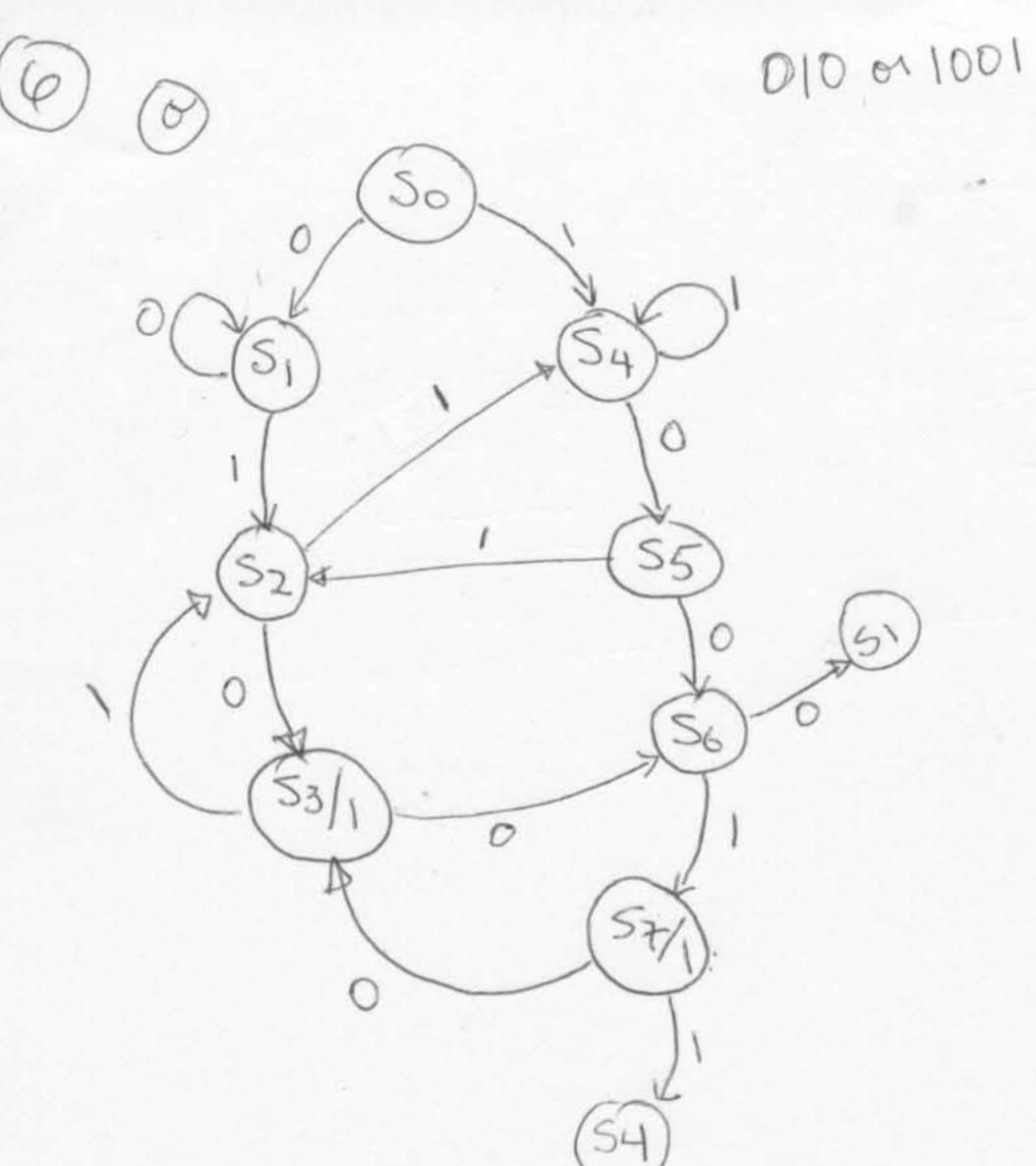
output next X=1 X=0 S4 SI 0 So 0 52 SI SI 52 0 SE 54 56 53 S2 - 1 S4 S5 0 S4 S2 0 56 55 0 S7 SI 56 57 54 53 the are no equivalent states
