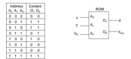
5. On the diagram shown below, specify and label the external connections that you would use to construct a 2-bit subtractor using two ROMs like the one developed in problem 4. The new circuit should accept two 2-bit numbers x1x0 and y1y0 and a borrow input bin. The output should be a 2-bit difference d1d0 and a 1-bit borrow bout. You should write on the diagram where would the input and output bits are to be connected and also how to connect the first ROM borrow output to the second ROM.
