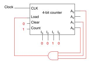
7. The stimulus program shown below is used to simulate the binary counter with parallel load described in the module named "counter". Going over the program, predict what would be the output of the counter and the carry output from t=0 to t=155ns.
