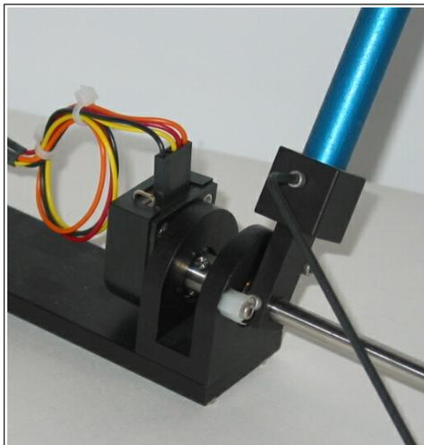
*Figure 4 - Tightening the setscrew*
