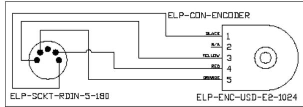
Schematic 1 Encoder Wiring
