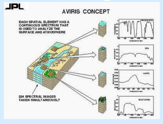
We can identify what is present in the image due to the spectral signature. NOTICE ONE PIXEL IS BIG!
