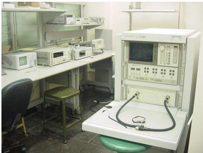
(b) Network Analyzer 8350 and other microwave equipment.
