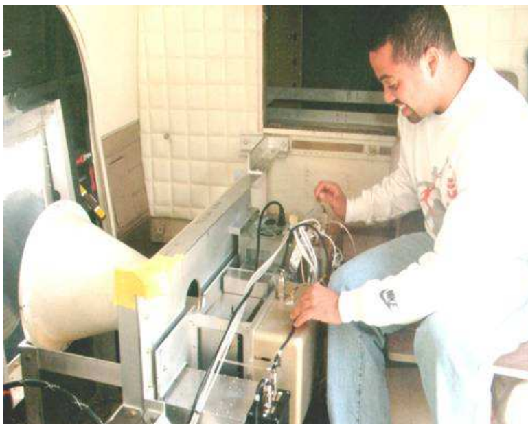
FIGURE. 3 UPRM STUDENT RAFAEL RAMIREZ PREPARING MM-WAVE RADAR FOR FLIGHT TEST, 1999
