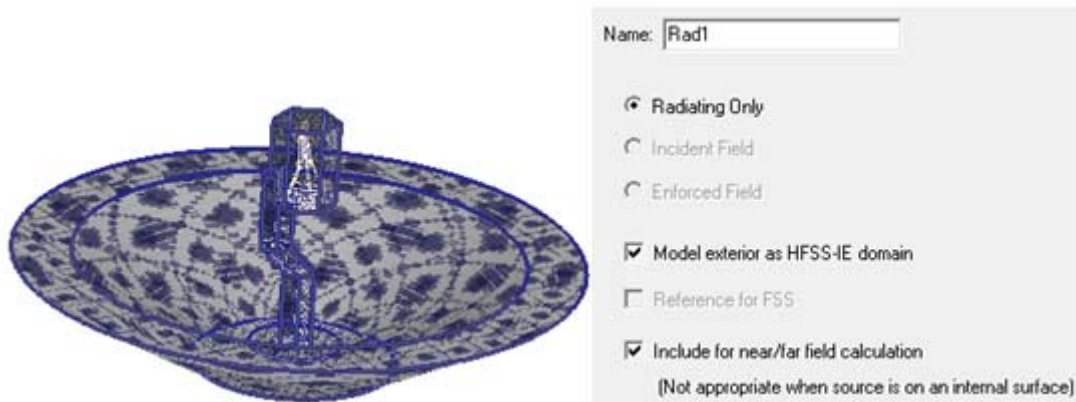
Figure 2: FEBI Boundary and Radiation Panel
