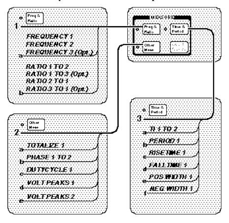
Figure 2-3. MEASURE Keys to SCPI Command Map (Part 1 of 2)
