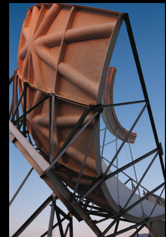
Antenna with no radome
