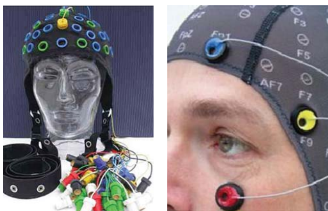
Figure 9.3 (Right) Electrode cap with built-in electrodes giving a specific montage. (Left) Electrode cap with many sites for individual screwed-in electrodes.
