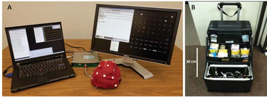
Figure 20.1 (A) The current Wadsworth P300-based BCI home system. The components include a laptop computer, an eight-channel EEG amplifier (Guger Technologies), an electrode cap (Electro-Cap International), a 20" monitor, and connecting cables. (B) A compact traveling BCI evaluation unit designed for easy setup, breakdown, and storage of all necessary hardware and supplies.
