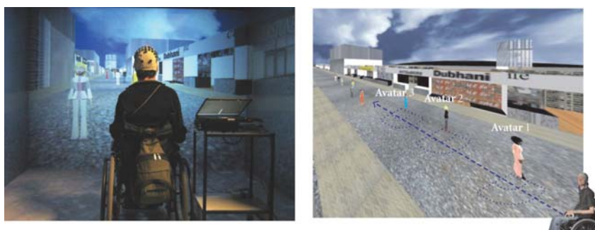
Figure 13.8 (Left) A virtual street populated with 15 avatars and a user with tetraplegia in his wheelchair in the middle of a multiprojection wall virtual reality system. The BCI user wore the electrode cap with one bipolar channel connected to the BCI system (amplifier and laptop on the right side). (Right) The task of the participant was to go from avatar to avatar in the direction of the end of the street (outlined with a dashed line). The avatars were lined up, and each avatar had an invisible communication sphere (drawn as dotted lines here). The BCI user had to stop within this sphere, not too close and not too far away from the avatar. (From Leeb et al., 2007.)
