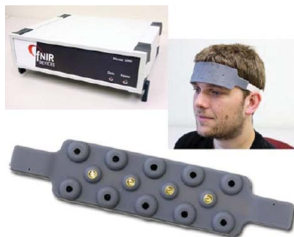
Figure 4.4 An example of an fNIRS device with sources and sensors. The four lights in the middle row are the illuminators, and the two rows at the edges house the 10 detectors. (Reprinted from Biopac Systems; retrieved from fNIRdevices.com .)
