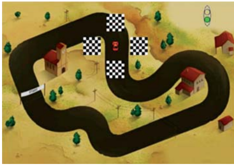
Figure 14.4 Screenshot of an SSVEP BCI to navigate a virtual car around a racetrack. The subject focuses on one of the four checkerboard patterns. Each of the 36 subfields switches between black and white at a different stimulus frequency. The four checkerboxes move with the car. (From Martinez et al., 2007.)
